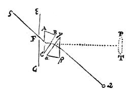
form; and all the fecond Prism, which refracts back again the rays to Q where the long image PT is contracted into a round one.
